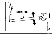
WARNING DO NOT turn the burners on when the cooktop is raised for cleaning. Be sure that the top is completely lowered and securely in place before turning on the burners.
