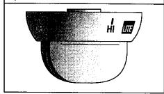
Each burner lights from either an electric ignitor or a standing pilot, depending on your model. Standing pilots must be lit initially. Refer to your installation instructions for instructions on lighting the standing pilot. Standing pilot will remain lit when the burners are turned off. Models with electric ignitors light automatically each time a control knob is turned to the LITE position.
