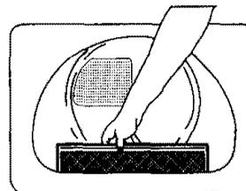
The Lint Filter is located in the bottom of the loading port and is accessible when the loading door is open. It filters all the air circulated through the dryer and traps the considerable
