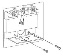
Position cord/conduit plate as shown in the following illustration.
