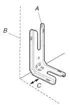
A. Anti-tip bracket B. Mark edge of range C. <sup>15</sup>/<sub>16</sub>" (2.4 cm)
