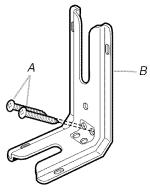
A. #12 x 15%" screws B. Anti-tip bracket
