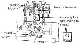
Follow the 3-wire power cord (option 5A), 3-wire conduit (option 5B) or 4-wire conduit (option 5C) sections as appropriate for your application.
