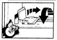
5. Slide bulb holder out, then turn towards front to remove bulb from oven.
