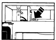
4. Remove bulb holder mounting screw.
