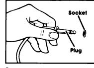
2. Place food in the oven and plug the probe into the socket on the oven wall.
