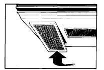
**4.** To replace grease filters, slide filter in the frame slot on the front of the opening.
