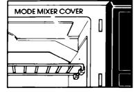
**NEVER** remove the mode mixer cover. The plastic cover protects the microwave mixer blade from soil or bending.
