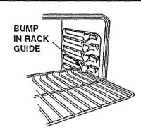
**NOTE:** The racks are designed with stop locks. When placed correctly on the rack support and extended from the oven, the stop lock prevents the racks from tilting when you are removing food from the racks or placing food on them.
