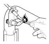
No adjustments are required for natural gas. If the range is connected to LP gas, contact the person who installed your range or made the conversion. If pilot flame does not stay lit, repeat this step.
