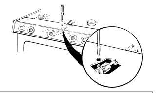
**CAUTION** – Make sure the surface burner control knobs are in the **OFF** position before attempting to adjust the pilots.
