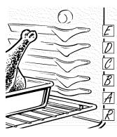
The oven has a special low shelf (R) position just above the oven bottom. Use it when extra cooking space is needed, for example, when cooking a large turkey. The shelf is not designed to slide out at this position.
