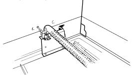
With the oven bottom removed, properly adjusted flames should have approximately 1" blue cones and, if range is supplied with natural gas, should burn with no yellow tipping. (With most LP gas, small yellow tips at the end of outer cones are normal.) Flames should not lift off burner ports. If lifting is observed, gradually reduce air shutter opening until flames are stabilized.
