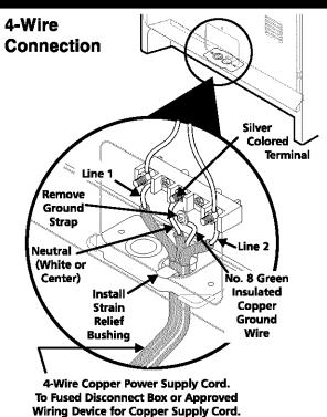
4. Using the nuts removed in step 1, connect the neutral (white) wire of the copper power supply cord to the center silver colored stud on the terminal block.
