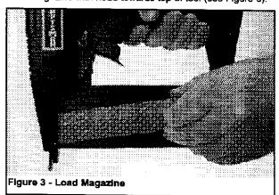
Slide magazine cover forward over magazine until latch snaps into place, locking magazine cover (see Figure 4).
