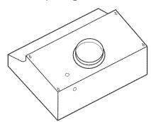
If roof or wall cap does not have a damper, install damper (supplied with hood) in vent system to prevent air from flowing back into vent system.
