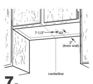
**To wire through top,** mark a line 7-1/2" from the right of the centerline on the underside of the cabinet. Mark the point on this line that is 2" from back wall. Drill a 1-1/4" diameter hole through the cabinet at this point. Note: If a cord-connection kit is used, drill a 1-5/8" diameter hole.
