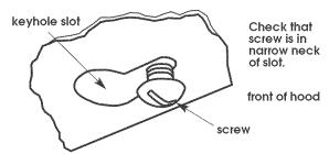
Lift range hood into final position, feeding electrical wire through wiring opening. Tighten mounting screws to cabinet, making sure mounting screws are in narrow neck of slot.
