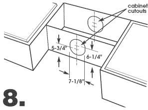
To vent through the roof or wall, mark 5-3/4" and 6-1/4" in from back wall along the centerline on underside of cabinet. Use these points as centers to draw 7-1/8" circles on underside of cabinet.
