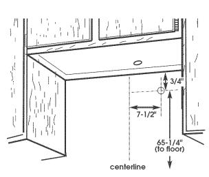
To wire through rear, mark a line 7-1/2" from the right of the centerline on the wall. Mark the point on this line that is 65-1/4" from the floor (or 3/4" from underside of cabinet). Drill a 1-1/4" diameter hole through wall at this point.
