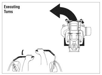
Figure 14. Turning Around a Corner
