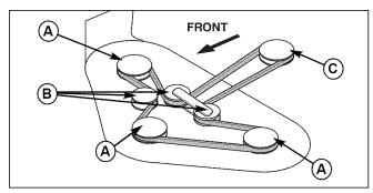
Figure 17. Mower Belt Routing
