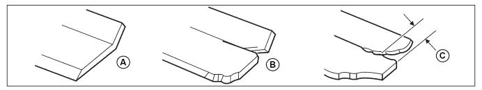
Figure 27. Inspecting the Mower Blade Air Lifts
