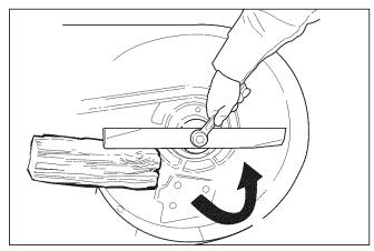
Figure 25. Loosening the Mower Blade for Removal
