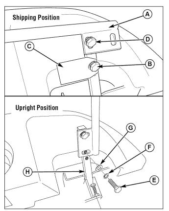
Figure 3. Install Control Levers (Left Side Shown)
