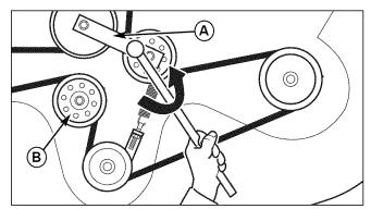
Figure 18. Release Belt Tension
