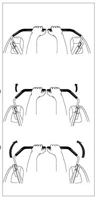
Figure 11. Move Control Levers Gradually
