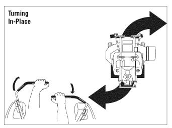
Figure 15. Turning in Place
