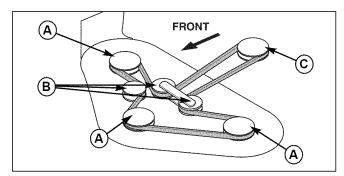
Figure 45. Mower Belt Routing
