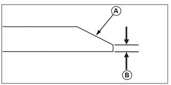
Figure 28. Sharpening the Mower Blade
