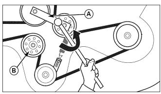
Figure 44. Release Belt Tension
