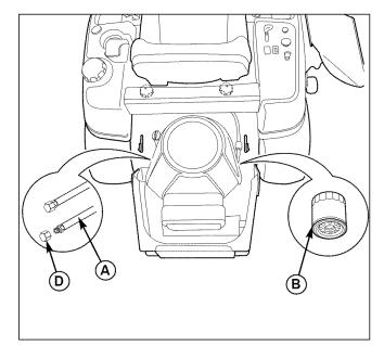
Figure 32. Change Engine Oil & Filter
