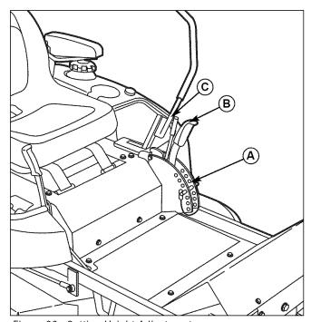
Figure 36. Cutting Height Adjustment
