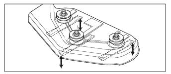
Figure 43. Orient Blades Front-to-Back
