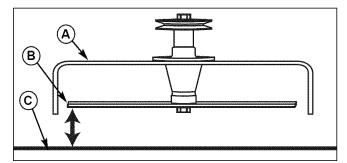
Figure 41. Measure Blade Tips to Ground
