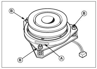
Figure 38. PTO Clutch Adjustment
