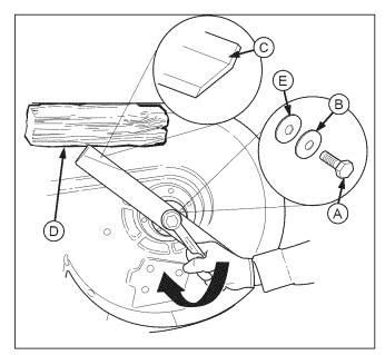
Figure 30. Tightening the Mower Blade for Installation
