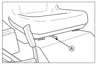
Figure 6. Seat Adjustment A. Adjustment Lever
