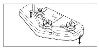
Figure 40. Orient Blades Side-to-Side
