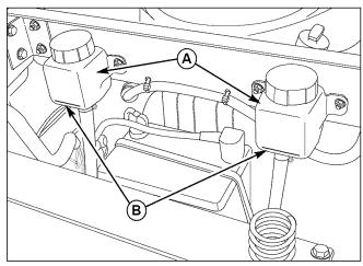
Figure 33. Transmission Oil Reservoirs
