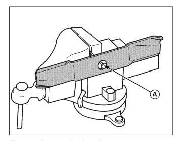
Figure 29. Balancing the Mower Blade A. Nail
