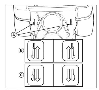
Figure 10. Transmission Release Levers
