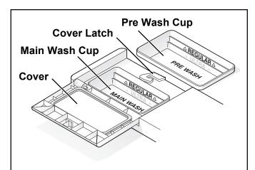
Note: If the cover is closed on the Main Wash Cup, open by pressing the cover latch.
