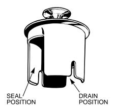
**To fill sink,** insert stopper so the *largest* slot lines up with the switch plunger. Stopper can now be pushed down to seal position without activating disposer.
