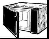
DO NOT operate the oven if it is damaged. It is particularly important that the oven door close properly and that there is no damage to the (1) Door (bent). (2) Hinges and latches
