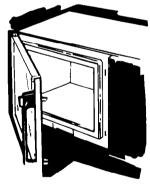
**NEVER** start a microwave oven when it's empty. The oven can be damaged. If you experiment, put a container of water in the oven.
