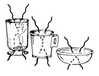
Microwaves pass through glass, paper and plastic without heating them so food absorbs the energy. Microwaves bounce off metal pans so food does not absorb the energy.
