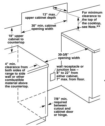
\*\* Note: 24" min. when bottom of wood or metal cabinet is protected by not less than 1/4" flame retardant millboard covered with not less than No. 28 MSG sheet steel, 0.015 stainless steel, 0.024" aluminum or 0.020" copper.
