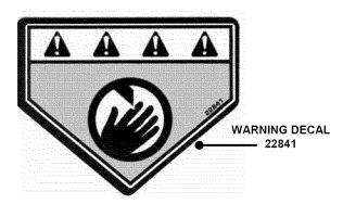
(4) WARNING: Located on the right side of the Mower Deck. It advises operator of the danger of the rotating blade.
