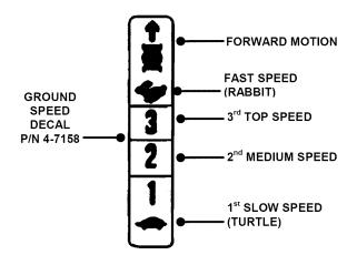
(7) GROUND SPEED: Shows direction of movement and the ability to select one of three ground speeds by moving the lever. The number 3 (Rabbit) indicates the top speed, number 2 indicates the medium speed and the number 1 (Turtle) indicates the slowest speed.
