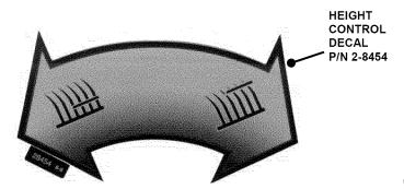
(8) HEIGHT CONTROL INSTRUCTION: Shows direction of movement of HEIGHT ADJUST HANDLE to select a change in height if cut from highest cutting height (clockwise) to the lowest height (counter-clockwise). Note that there is a total of eleven heights of cut.
