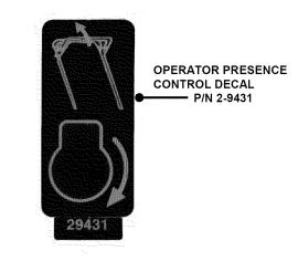
(11) **OPERATOR PRESENCE CONTROL:** Pull control against handle to start engine and blade. Release control to stop engine and blade.
