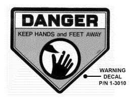
(15) WARNING: Located on the right side of the Mower Deck. It advises operator of the danger of the rotating blade.
