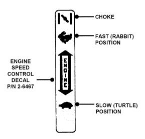
**(6) ENGINE SPEED CONTROL:** Indicates direction to increase Engine RPM (Rabbit), decrease Engine RPM (Turtle), and direction to choke.
