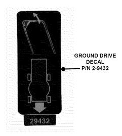
(12) **GROUND DRIVE:** Pull lever against handle to engage drive. Release lever to disengage drive.
