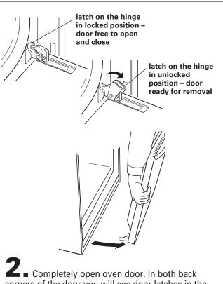
Completely open oven door. In both back corners of the door you will see door latches in the locked position. Rotate both latches forward to the unlocked position.
