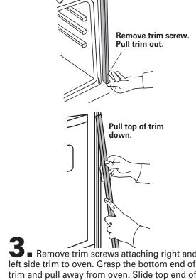
Remove trim screws attaching right and left side trim to oven. Grasp the bottom end of trim and pull away from oven. Slide top end of trim downward to remove trim from oven. Take care not to scratch other surfaces with ends of trim. Set trim and screws aside on protected surface.
