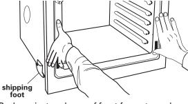
Push against seal area of front frame to push oven into cabinet until shipping feet almost contact cabinet. Use a Phillips screwdriver to remove screws attaching shipping feet. Remove and discard shipping feet.
