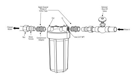
**Note:** Can be installed undercounter (as shown), in basement, or other convenient location. See installation instructions packed with product for complete details.
