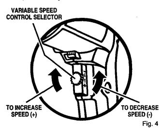
Note: Hold your hammer drill in normal operating position and turn the variable speed control selector clockwise to increase (+) the speed and torque of your hammer drill. Turn counterclockwise to decrease (-) the speed and torque of your hammer drill.
