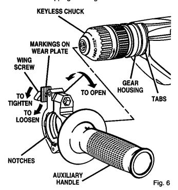
To prevent possible loss of control, auxiliary handle should be checked periodically for tightness. Do not operate hammer drill with auxiliary handle loose.
