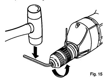
Unlock spindle by removing nail or pin from slot in gear housing.
