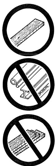
3. Rip only workpieces longer than the diameter of the blade. Do not rip workpieces that are shorter than the diameter of the blade being used.
