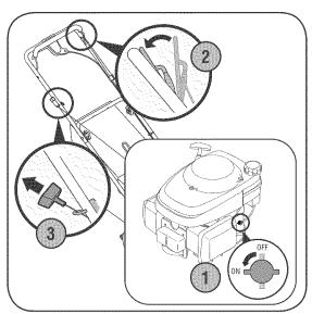
Figure 4-2: Starting the mower.
