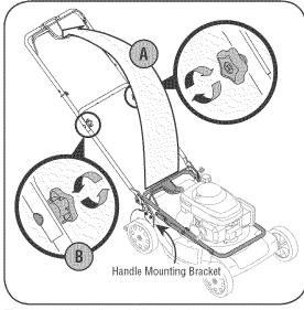
Figure 3-1: Lift handle and tighten hardware.
