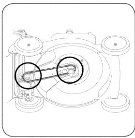
Figure 5-5: Remove belt from transmission and engine pulley.
