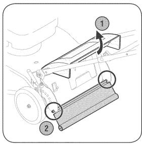
Figure 5-2: Replacing the rear flap.
