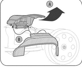
Figure 3-5: The mulching baffle
