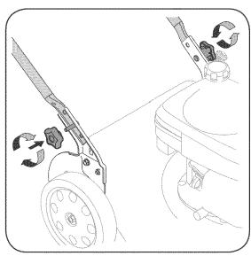
Figure 3-2: Secure handle to handle mounting brackets.
