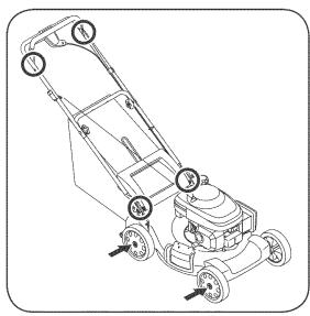
Figure 5-1: Lubrication areas on the mower.
