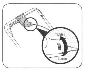
Figure 3-8: The adjustment wheel on the drive control.
