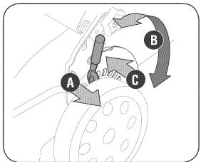
Figure 3-7: The cutting height adjustment lever.
