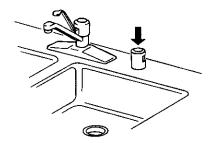
The drain air gap is usually located on top of the sink or countertop near the dishwasher. To order a drain air gap contact your local dealer, or in the U.S.A., call the Consumer Assistance Center at 1-800-422-1230 and ask for Part Number 300096.
