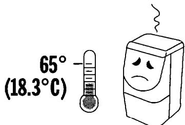
If ice forms on coils, some dehumidifiers will continue to cycle on and off. Some dehumidifiers have a de-icer feature that will automatically shut the dehumidifier off when ice forms. Unplug either type of dehumidifier until ice melts and room temperature rises.
