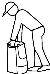
When moving dehumidifier, use the grip areas with both hands to push dehumidifier to a new location. Do not lift the dehumidifier with grip area. Pick dehumidifier up from the bottom to carry.
