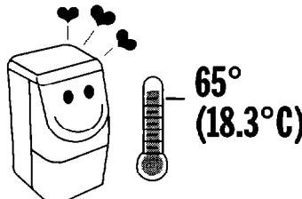
Install your dehumidifier in an area where the temperature will not fall below 65°F (18.3°C). Lower temperatures will cause ice to form on coils.
