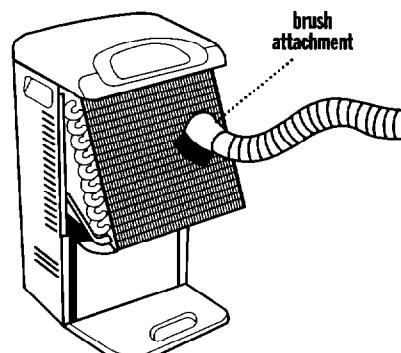
5. Clean coils with brush attachment of your vacuum cleaner. Be careful — coil fins are sharp.
