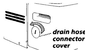
1. Use a flat-blade screwdriver to remove cover from drain connector. Turn cover counterclockwise. Discard cover. It cannot be reused.
