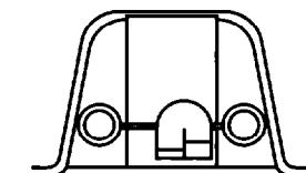
"Low" setting: Slide Water Level Float to "low" position—right side of opening — to make the bucket lighter to carry. The dehumidifier will shut off automatically when bucket is 1/2 full.
