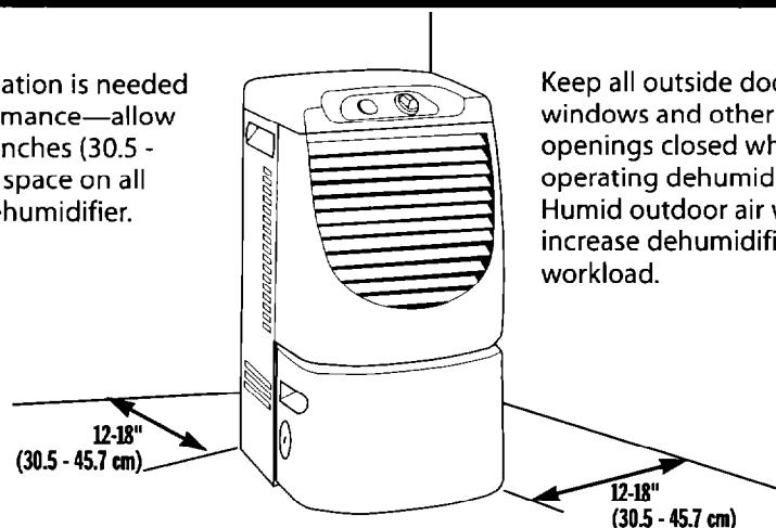
Keep all outside doors, windows and other openings closed when operating dehumidifier. Humid outdoor air will increase dehumidifier workload.
