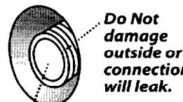
2. Drill out only the center of the drain hose connector. Use a minimum 1/4" drill bit.
