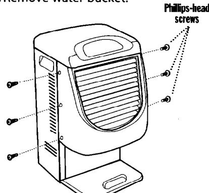
3. Remove 3 screws from each side of the front panel.
