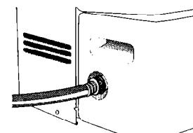
3. Attach a garden hose to drain hose connector. The garden hose should not be longer than 8 feet (2.4 m). Run other end of garden hose into a floor drain. Check that the hose lies flat and in the drain.
