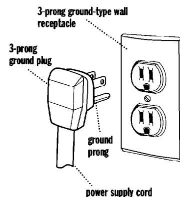
For your personal safety, this dehumidifier must be grounded. This dehumidifier is equipped with a power supply cord having a 3-prong ground plug.
