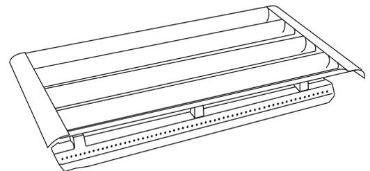
Check to be sure all burners are in the correct position. Burners should rest flat over the anti-flip brackets with stubs on top and flat side down.
