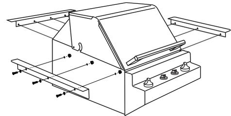
**NOTE:** This trim kit is not designed to support the weight of the grill. The grill must be supported from the bottom.
