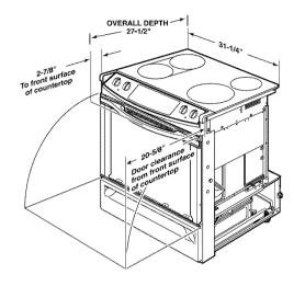
**NOTE:** The oven below the cooktop meets UL requirements for 0" clearance to back and side walls and cabinets.
