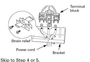
For conduit installations only, purchase a squeeze connector matching the diameter of your conduit and assemble it in the hole. Insert the conduit through the squeeze connector and tighten. Allow enough slack to easily attach the wires to the terminal block.
