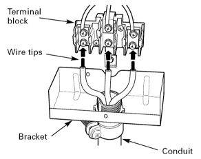
Wire used, location and enclosure of splices, etc., must conform to good wiring practices and local codes.
