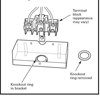
C For power cord installations only (see the next step if using conduit), assemble the strain relief in the hole. Insert the power cord through the strain relief and tighten. Allow enough slack to easily attach the cord terminals to the terminal block. If tabs are present at the end of the winged strain relief, they can be removed for better fit.
