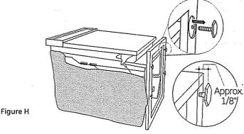
Screw leveling legs back into the dishwasher frame, approximately 1/8" from frame as shown.
