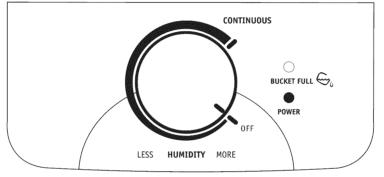
To turn the unit on rotate the knob until it points to the CONTINUOUS setting. It is recommended you leave the unit running in the CONTINUOUS setting for the first three or four days until any sweating and dampness odors have ceased.
