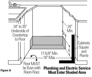
• The rough cabinet opening must be at least 24" deep and 17-5/8" to 18" wide. The opening should be 34" to 35" max. height.
