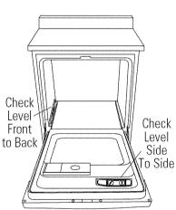
• Level the dishwasher by adjusting the four leveling legs individually.
