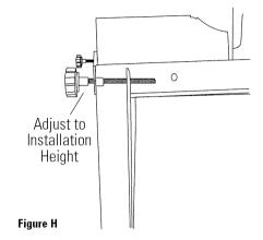
• Measure installation height and dishwasher height. Extend leveling legs out from the dishwasher base, 1/4" less than installation height.
