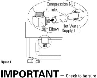
**INPORIANI** — Check to be sure that door spring does not rub or contact the fill hose or water supply line. Test by opening and closing the door. Re-route the lines if a rubbing noise or interference occurs.
