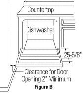
**Note:** ADA installation, (32-1/2") beneath 34" high countertops may be accomplished by adjusting the toekick and leveling legs.
