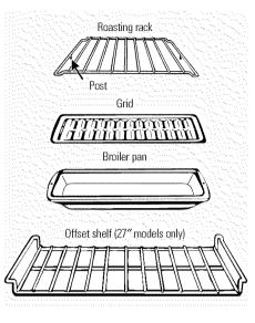
Place the meat on the special roasting rack. The rack holds the meat. The rack allows the heated air to circulate under the meat and increase browning on the underside of the meat or poultry.
