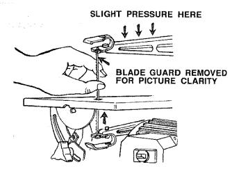
3. Look at the blade holders closely and notice the blade slots and pin recesses in the blade holder. The blade holder is made so you can position the blade for cutting from the front or one side of the saw.
