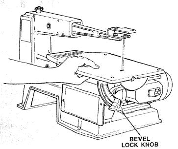
2. Use a small square to set the table at 90° to the blade. If there is too much space between the square and the blade, the table must be adjusted.
