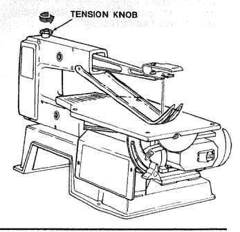
Remove blade by pulling forward on blade and then lifting the blade through the access hole in the table.
