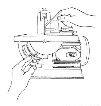
4. Loosen the screw holding the bevel scale pointer and adjust to 0°. Tighten screw.
