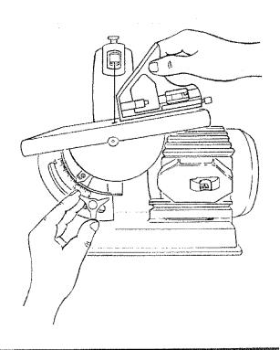
3. When the space between the square and the blade is minimal, tighten the bevel lock knob.
