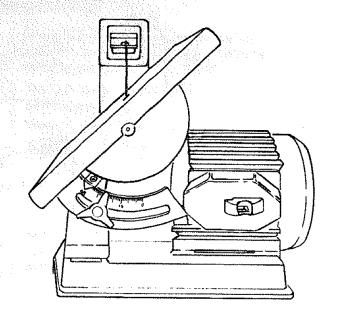
2. A bevel scale is provided under the work table as a convenient reference for setting the approximate table angle for bevel cutting.
