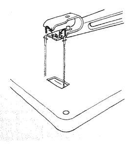
4. Locate the blade guard and carefully install it onto the saw as shown.
