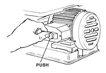
4. To lock switch in "OFF" position, hold switch IN with one hand, REMOVE key with other hand.
