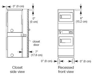
Additional clearances for wall, door and floor moldings may be required or if external exhaust elbow is used.
