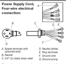
Four-wire power supply cord must have four, No.-10 copper wires and match a four-wire receptacle of NEMA Type 14-30R. The fourth wire (ground conductor) must be identified with a green cover and the neutral conductor by a white cover. 5. Remove the center terminal block screw.
