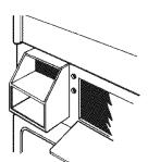
Secure coin slide mechanism from inside the control panel using the ¾6" bolt and washer included with the slide mechanism. Install coin box.
