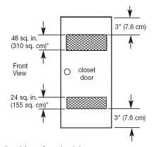
\*Opening is the minimum for a closet door. Louvered doors with equivalent air openings are acceptable.
