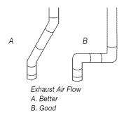
Allow as much room as possible when using elbows or making turns. Bend vent gradually to avoid kinking.
