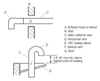
Do not install screening or cap over the end of the vent.
