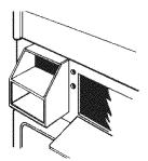
Secure coin slide mechanism from inside the control panel using the <sup>3</sup>/<sub>16</sub>" bolt and washer included with the slide mechanism. Install coin box.
