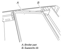
3. To remove the broiler pan, tilt the broiler pan and lift it out from between the supports.
