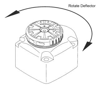
Figure 4 - Exhaust Deflector Adjustment
