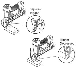
Figure 3 -Contact Trip Operation
