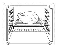
Use the convection roasting rack on the broiler pan and grid (all included with your oven). (The convection roasting rack rests on the broiler pan and grid.) The long side of the rack should be parallel with the oven door for best heat distribution and airflow.
