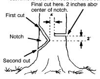
After removing the cutout of wood, make the felling cut on the opposite side of the notch. This is done by making a cut about two inches higher than the center of the notch. This will leave enough uncut wood between the felling cut and the notch to form a hinge. This hinge will help prevent the tree from falling in the wrong direction.
