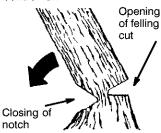
NOTE: Before felling cut is complete, use wedges to open the cut when necessary to control the direction of fall. Use wood or plastic wedges, but never steel or iron, to avoid kickback and chain damage.
