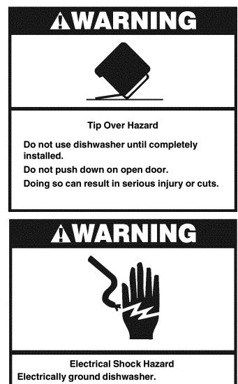
Connect ground wire to green ground nut in terminal box.
