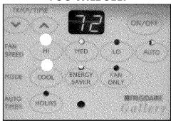
Note: Tap or hold either  $up(\land)$  or  $down(\lor)$  button until the desired temperature is seen on the screen. This temperature will be automatically maintained anywhere between 60F (15C) and 90F (32C). If you want the display to read the actual room temperature, see step 5.
