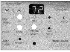
Note: In this mode, when the compressor shuts off, the fan will continue to run for another 3 minutes, then shut off until cooling is needed, as sensed by the room temperature control. During this time, it may come on for 3 minutes to sense whether cooling is needed, then it will go off for 15 minutes. It will continue doing this to sample the room air for as long as necessary.
