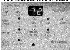
Note: Tap or hold the UP arrow(^) to increase delayed start time by .5 hours (up to 10 hours), then in 1 hour increments up to 24 hours. The control will count down the time remaining until start (8, 7.5, 7, etc.).
