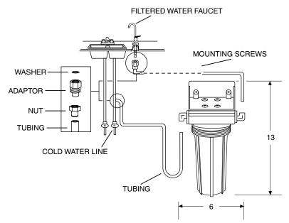
Note: Can be installed undercounter (as shown), in basement, or other convenient location. See installation instructions packed with product for complete details.
