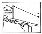
After replacing with same size bulb, reinstall panel (hang top on pins; pull bottom down, push it back and release it to let lip engage grooves in retainers).
