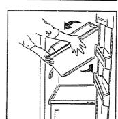
7. Pull the drawer forward, lift the front to clear stops, and pull the drawer out until it hits the door. Then lift the drawer up until it is higher than the drawer supports, tilt it and take it out.
