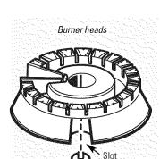
The burner heads are removable. Simply lift them off the range for cleaning.
