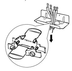
**NOTE:** The replacement power cord must be a 3-conductor or a 4-conductor UL-listed range cord or conduit. Cords may be provided with ring terminals on wire and a strain relief device.
