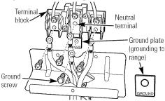
Place the terminal screws and ground screw in safe location for later use.
