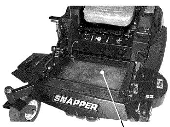
LIFT FOOT REST UP AND OFF POWER UNIT FRAME TO GAIN ACCESS TO MOWER BELT
