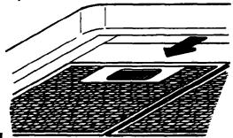
■ Press on handle in front of filters to release filters from range hood canopy. Remove filters and set aside.
