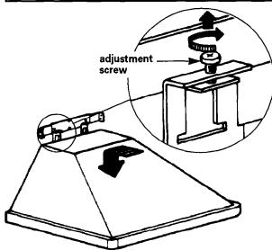
Rotate the two adjustment screws halfway into slots. Hang canopy from flange of lower bracket, making sure that tabs are fully inserted in slots and canopy is secure on bracket. Adjust the height of the canopy by rotating the two screws.
