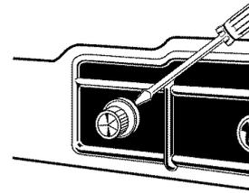
3. Unplug burned out signal light and replace it with a new one.
