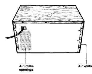
3. Do not block the rear air intake openings and air vents on side of microwave oven. Allow a few inches of air circulation on side and back of oven where vents and intake openings are located. Blocking the air intake openings and air vents can cause damage to the oven and poor cooking results. Make sure the microwave oven legs are in place to ensure proper airflow.
