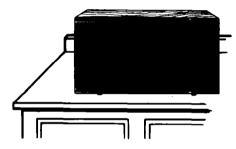
Put the oven on a cart, counter, table or shelf that is strong enough to hold the oven and the food and utensils you put in it. (The control side of the unit is the heavy side. Use care when handing.) The weight of the oven is approximately 33 lbs (15 kg).
