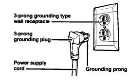
It is the personal responsibility and obligation of the customer to have a properly grounded and correctly polarized 3-prong wall receptacle installed by a qualified electrician.
