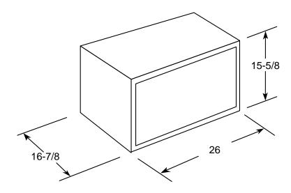
**Note:** When installing units in through-the-wall applications. Do not restrict air flow areas.
