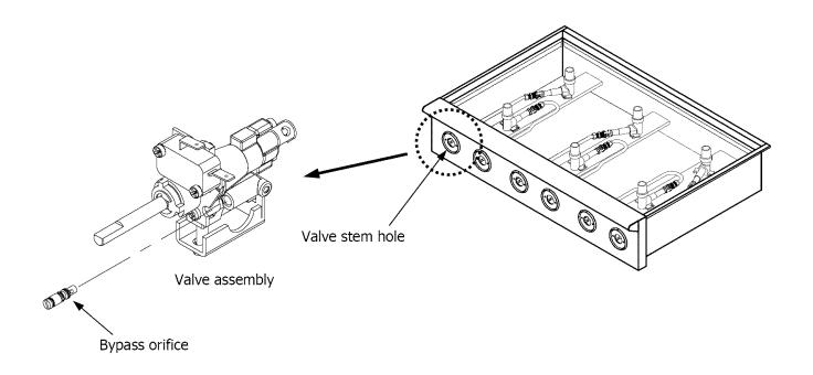
Figure 6-1 Bypass Orifice Conversion
