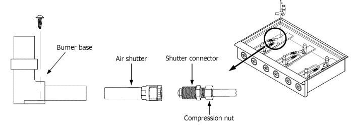
Figure 9-1 Air Shutter Assembly
