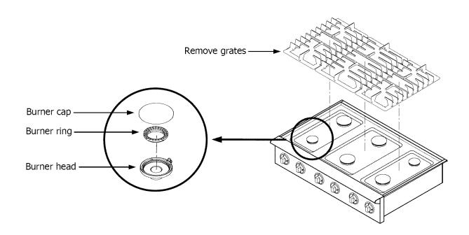
Figure 3-1 Grate, Burner Cap, and Burner Ring Removal
