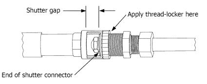
Figure 9-2 Air Shutter Reassembly and Gap Adjustment
