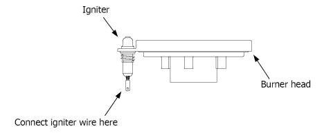
Figure 10-1 Igniter Location and Connection
