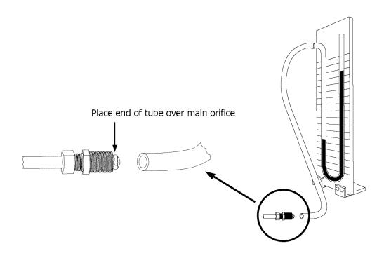
Figure 8-1 Pressure Test Set-up
