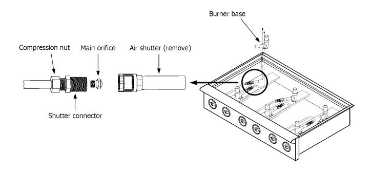
Figure 7-1 Main Orifice Conversion
