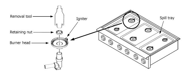
Figure 5-1 Burner Head Removal
