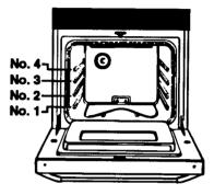
Each oven has two racks. One rack is straight and the other is offset (raised). The shape of the offset rack helps you space racks better.
