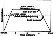
The Self-Cleaning cycle uses very high heat to burn away soil and grease. During the cycle, the oven gets much hotter than it does for normal baking or broiling. This high heat breaks up the soil or grease and burns it away. Your oven is preset for a 3-hour Self-Cleaning cycle. However, you can adjust the cycle time to the amount of soil in your oven. You can set the cycle anywhere between 2 and 4 hours. (See "Setting the controls" on page 31.)
