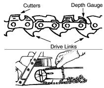
Place chain onto the sprocket
