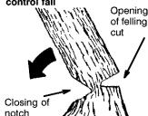
NOTE: Before felling cut is complete, use wedges to open the cut if necessary to control the direction of fall. To avoid kickback and chain damage, use wood or plastic wedges, but never steel or iron wedges.
