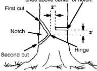
After removing the wood from the notch, make the felling cut on the opposite side of the notch. This is done by making a cut about two inches higher than the center of the notch. This will leave enough uncut wood between the felling cut and the notch to form a hinge. This hinge will help pre-vent the tree from falling in the wrong direc-
