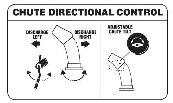
The chute directional control is located on left side of the snow thrower. To change the direction in which snow is thrown, turn chute directional control as follows:
