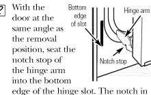
edge of the hinge slot. The notch in the hinge arm must be fully seated into the bottom of the slot.
